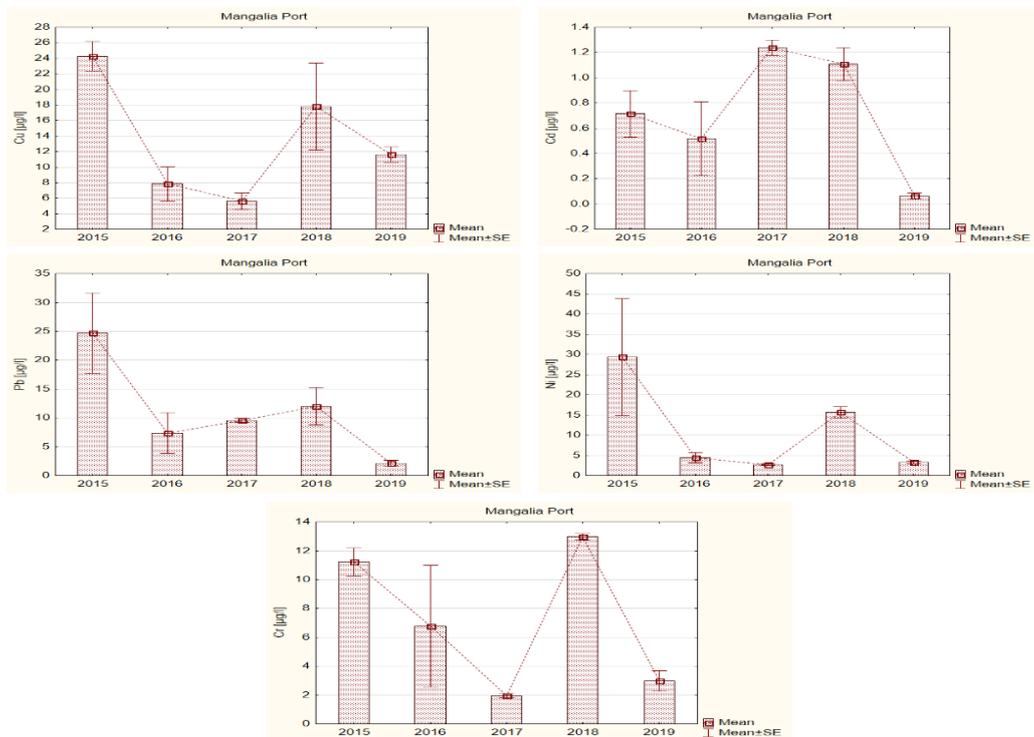
Figure 2.58 - Trends of heavy metals concentrations in surface waters - Mangalia Port area, 2015 - 2019
