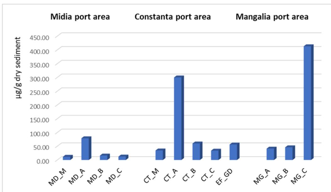
Figure 3.48 - Spatial distribution of TPHs concentrations in surface sediments in hot-spots study areas, September 2019
