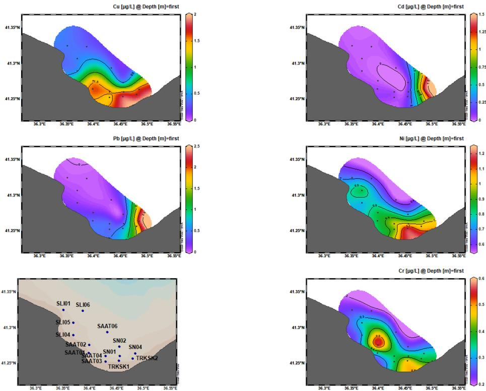
**Figure 2.70 - Special distribution of the metals in water collected from Samsun Hot Spot area, summer 2019**
