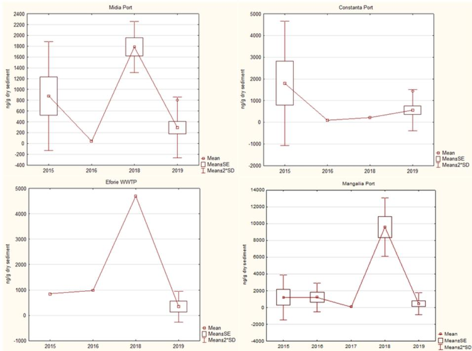
Figure 3.51 - Trends of total PAHs concentrations in surface sediments in Midia, Constanta, Eforie and Mangalia areas, 2015 - 2019
