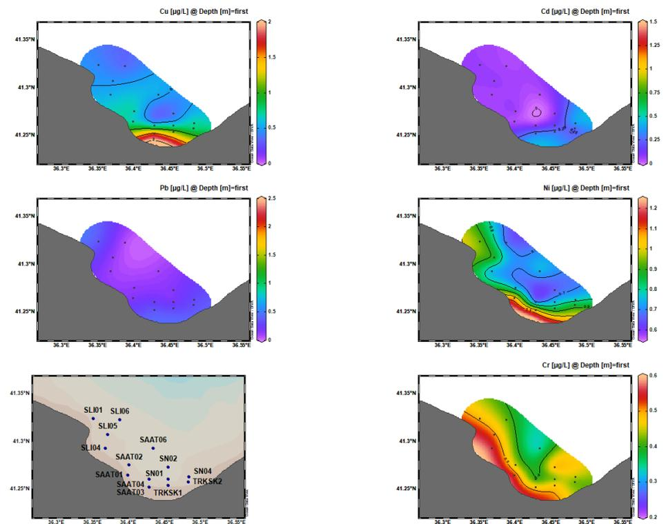
**Figure 2.71 - Special distribution of the metals in water collected from Samsun Hot Spot area, winter 2020**
