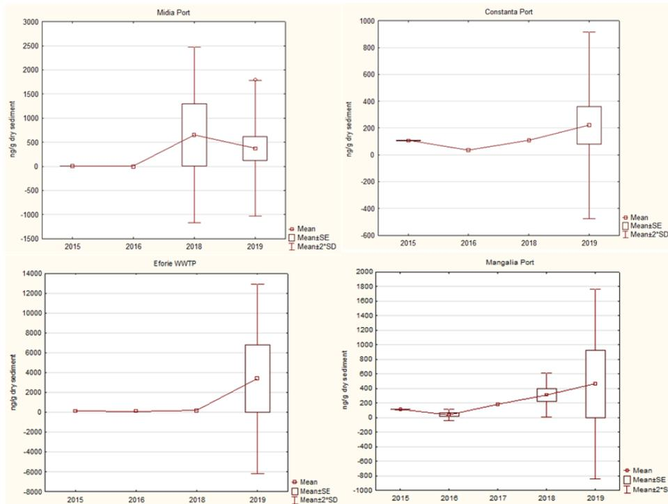
**Figure 3.49 - Trends of total OCPs concentrations in surface sediments in Midia, Constanta, Eforie and Mangalia areas, 2015 - 2019**
