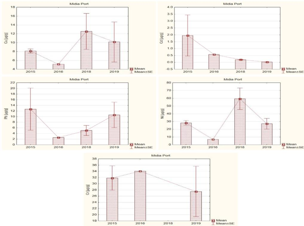
**Figure 3.43 - Trends of heavy metals concentrations in surface sediments inside and surrounding area - Midia Port, 2015 - 2019**
