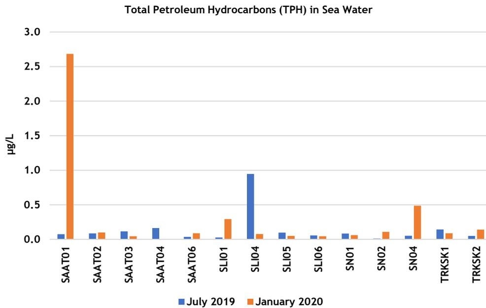
**Figure 2.74 - TPH concentrations in seawater, Samsun Hot Spot**
